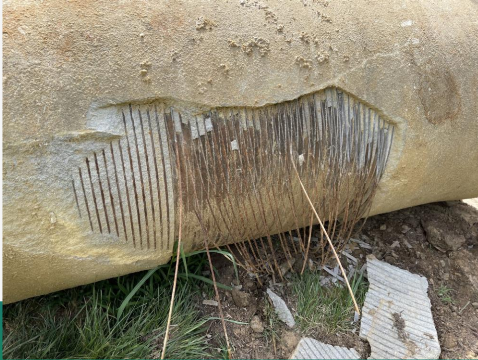
36" PCCP with Severely Corroded and Broken Pre-Stressed Wires
